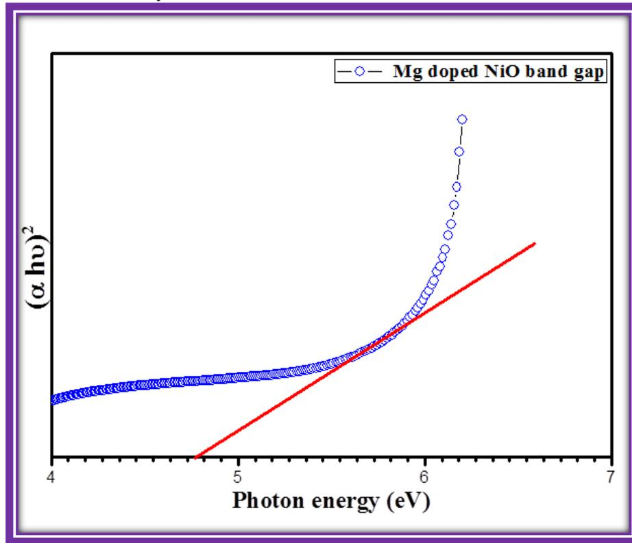
**Figure 6: Band Spectrum of Mg<sup>2+</sup> doped NiO nanoparticles**
