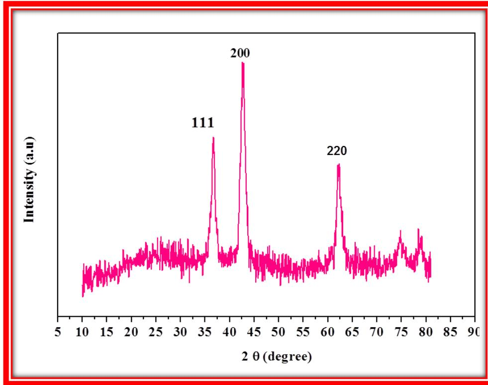
**Figure 1: XRD pattern of Mg<sup>2+</sup> doped NiO Nanoparticles**
