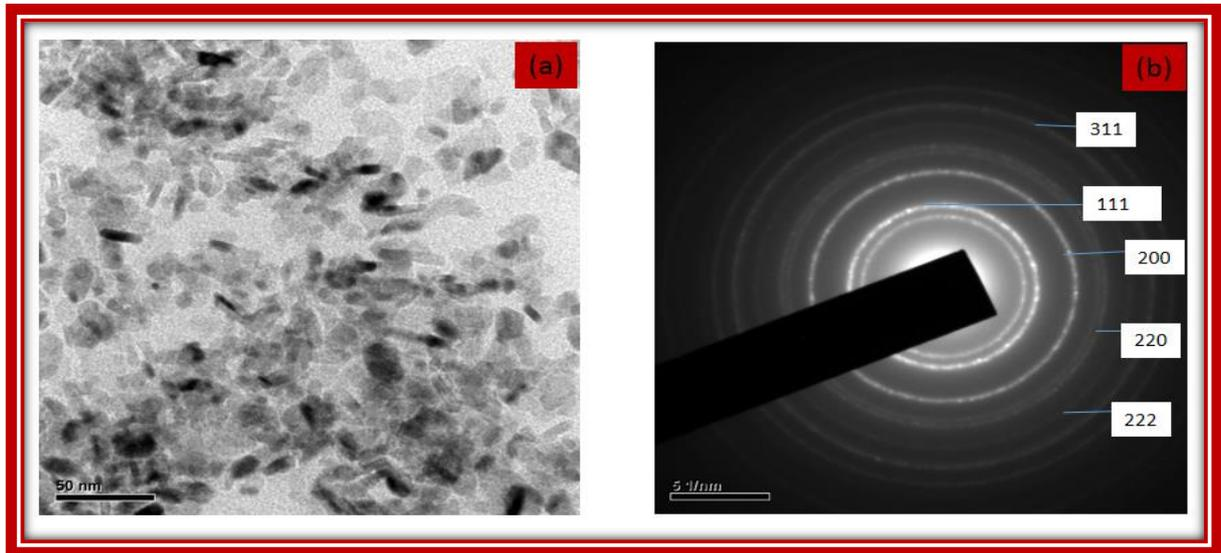
**Figure 2 (a) HRTEM image Figure 2 (b) SAED studies of Mg<sup>2+</sup> doped NiO nanoparticles**
