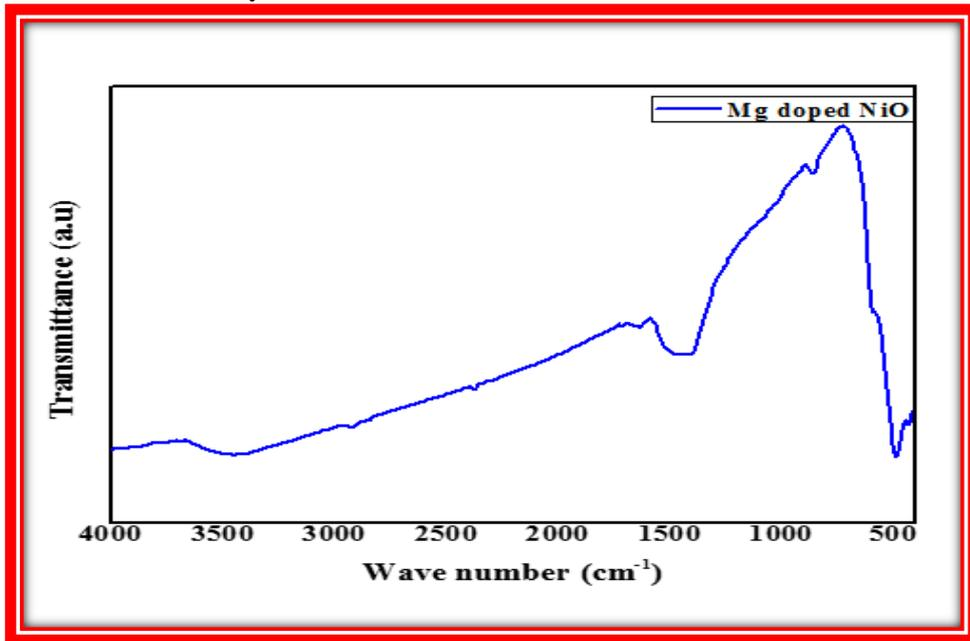
Figure 4. FTIR spectrum of Mg<sup>2+</sup> doped NiO nanoparticles
