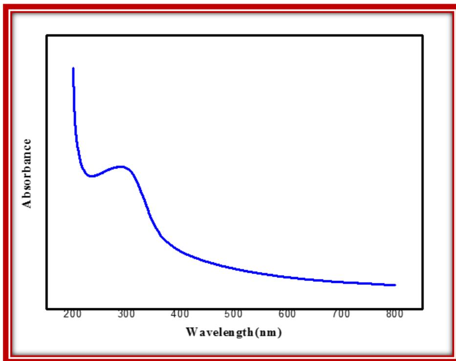
Figure 5. UV-vis spectrum of Mg<sup>2+</sup> doped NiO nanoparticles
