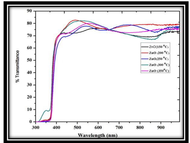
Figure 5. Plot of % transmittance versus wavelength (nm) of ZnO thin films
