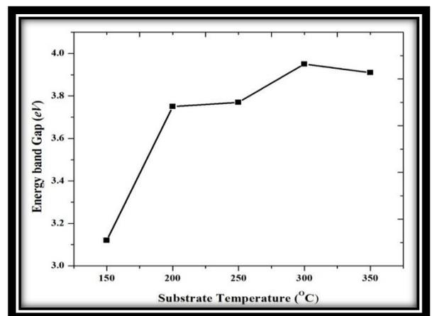
Figure 7. Variation of band gap energy versus substrate temperature
