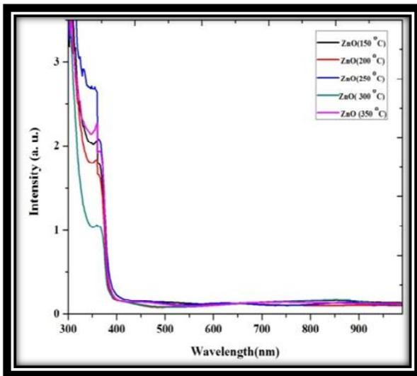
Figure 4. The Absorption Spectra of ZnO thin Films
