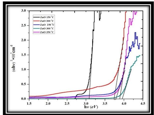
Figure 6. Tauc Plot of ZnO thin films reported in earlier study [13]. The film deposited at 300 °C substrate temperature exhibit higher band gap (3.95 eV).
