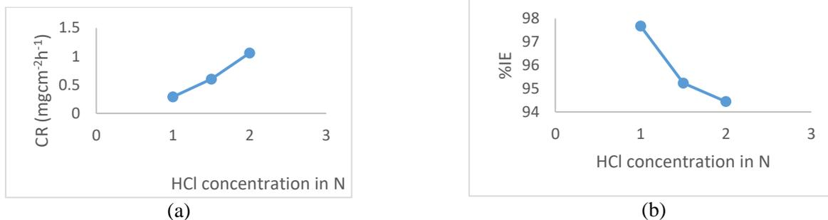
**Fig 2. (a) Change of Corrosion Rate and (b) Change of % Inhibition Efficiency of Inhibitor I in 200 ppm ] Concentration with Different Concentration of HCl**
